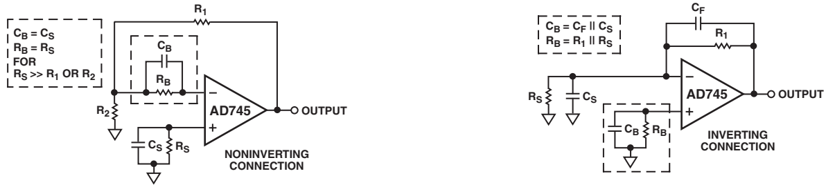
Figure 40. Optional External Components for Balancing Source Impedances
