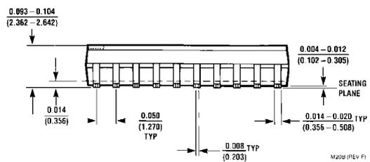
**20-Lead Small Outline Integrated Circuit (SOIC), JEDEC MS-013, 0.300" Wide
