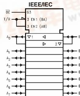
74LVT245 • 74LVTH245 Low Voltage Octal Bidirectional Transceiver with 3-STATE Inputs/Outputs
