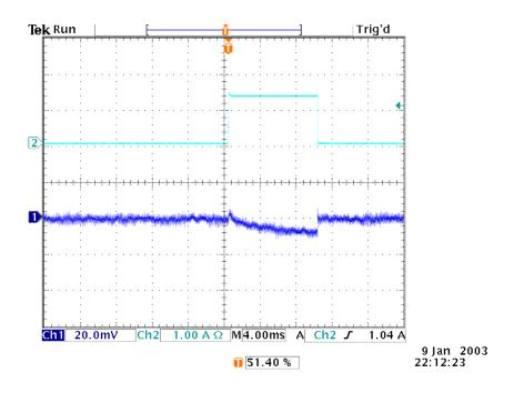
W83310S-N  $V_{TT}$  offset with a 1.5A/10ms sinking pulse current.
