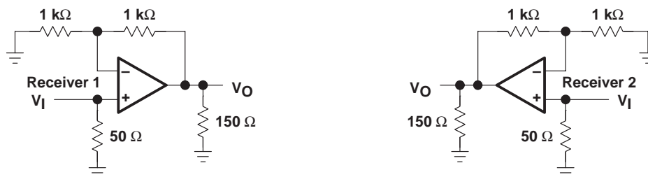
Figure 2. Receiver Input-to-Output Crosstalk Test Circuit
