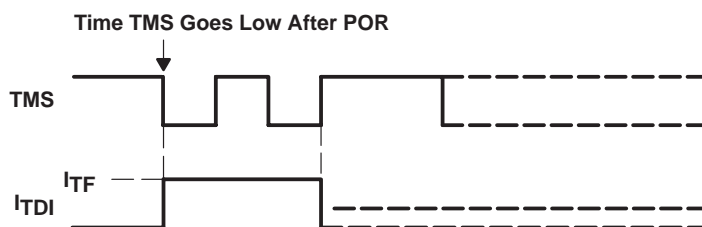
Figure 8. Fuse Check Mode Current, MSP430P/E325A, C32x
