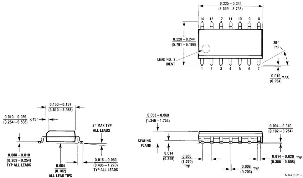
**14-Lead Small Outline Integrated Circuit (SOIC), JEDEC MS-120, 0.150 Narrow
