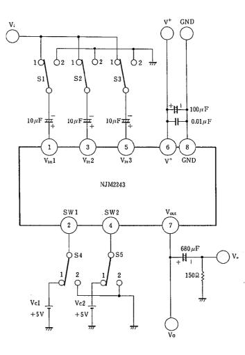
DC Voltage Each Terminal Typ. on Test Circuit Ta =25℃
