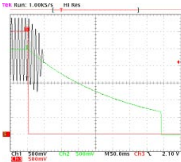
Figure 40. Turning-Off Time/ V_p = 5.0 V and F = 100 Hz Ch1 = OUT_R, Ch2 = VMC and Ch3 = Shutdown
