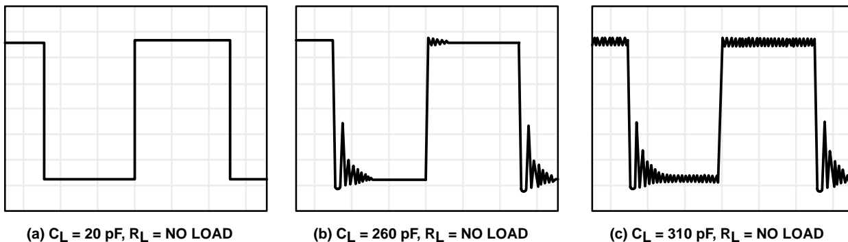
Figure 112. Effect of Capacitive Loads in Low-Bias Mode
