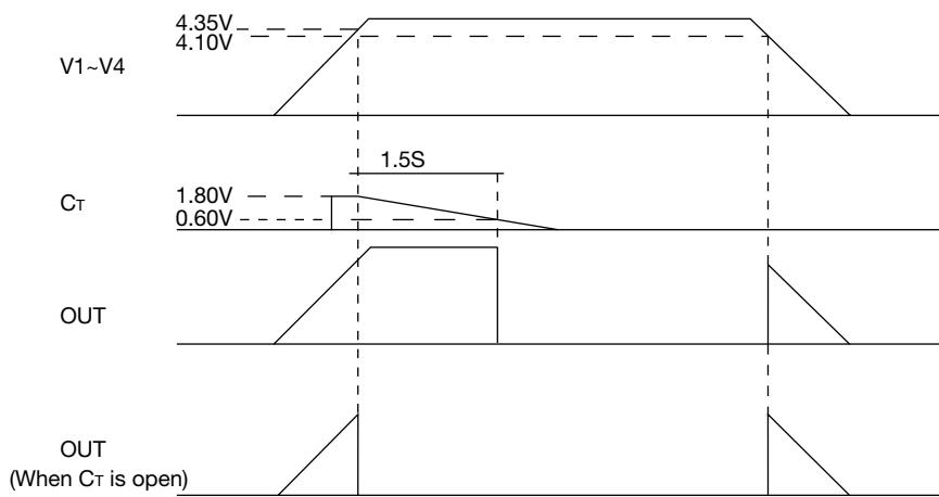
Note : When pin Ct is shorted or left open, the output goes low when overcharging is detected.
