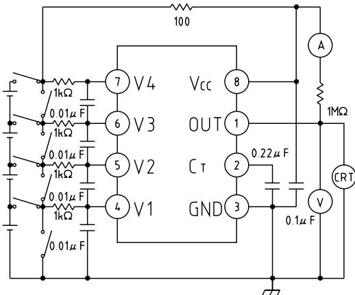
Note 1: By shorting each cell, two-, three- and four-cell series can be accommodated. A V4 cell should always be connected. If the V4 cell is shorted, the chip may not function correctly.
