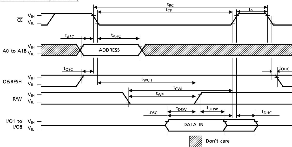
WRITE CYCLE 2 (OE CLOCKED & LOW)
