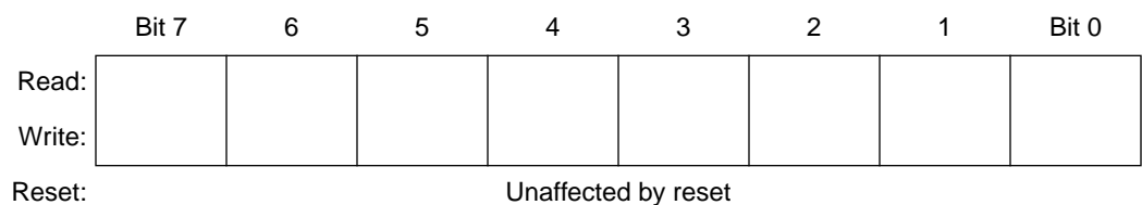
Figure 13. Index Register (X)
