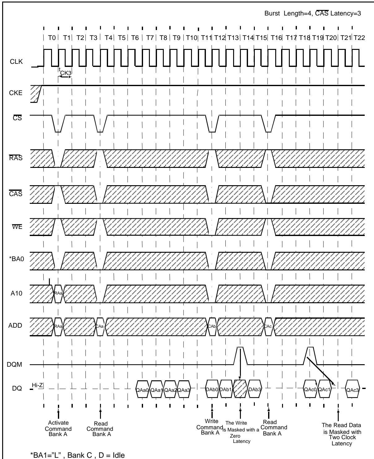
**Interleaved Column Read Cycle (1 of 2)**
