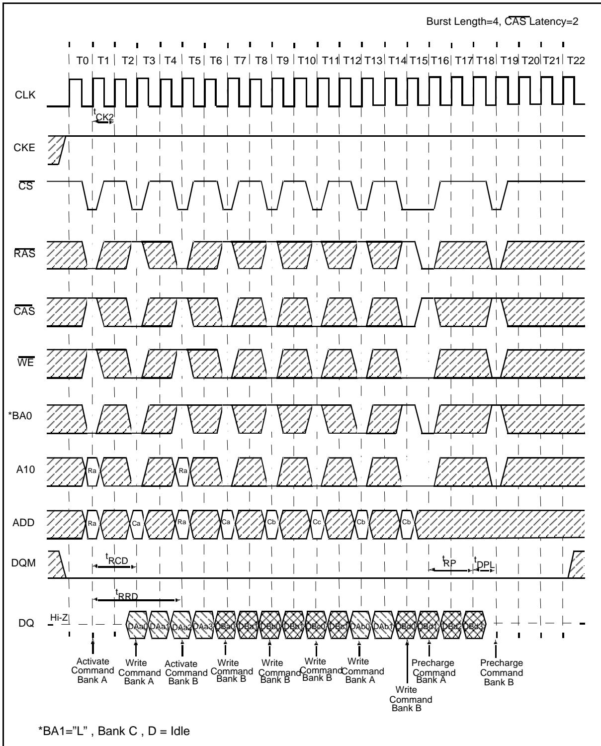
**Interleaved Column Write Cycle (2 of 2)**
