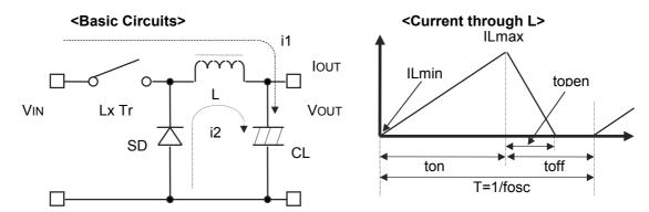
Step 1: Lx Tr. turns on and current IL (=i1) flows, and energy is charged into CL. At this moment, IL increases from ILmin. (=0) to reach ILmax. in proportion to the on-time period(ton) of LX Tr.
