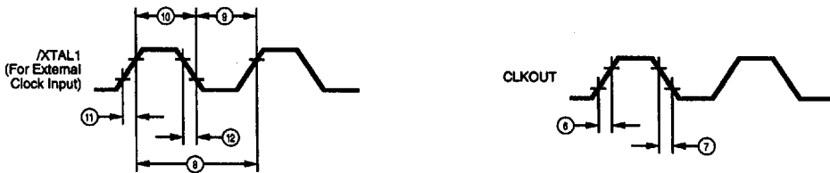
(a) XTAL1 Timing for External Clock Input
