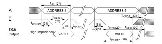
v: Ē must be used to clock in the address sequence for the software controlled STORE and RECALL cycles.
