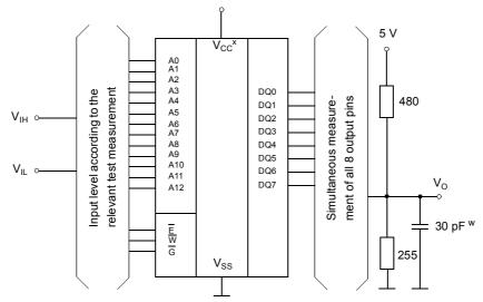
w: In measurement of  $t_{\text{dis}}\text{-times}$  and  $t_{\text{en}}\text{-times}$  the capacitance is 5 pF.
