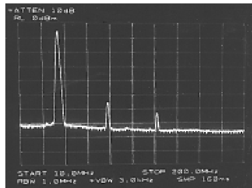
Figure 48. Output Spectrum of Enhanced Dynamic Range Circuit (Output Level = 61 dBmV, Frequency = 42 MHz)
