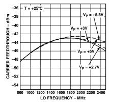
Figure 9. Carrier Feedthrough vs.  $F_{LO}$ . LO input level = -10 dBm.
