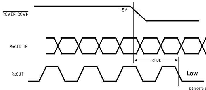
**FIGURE 10. DS90CF384A/DS90CF364A (Receiver) Power Down Delay**
