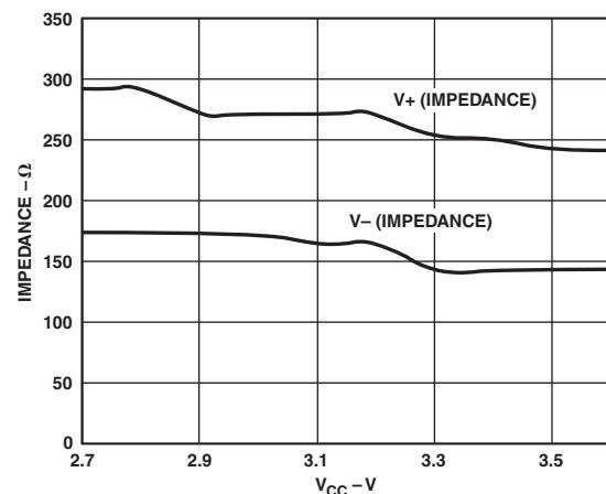
TPC 5. Charge Pump Impedance vs. V<sub>CC</sub>
