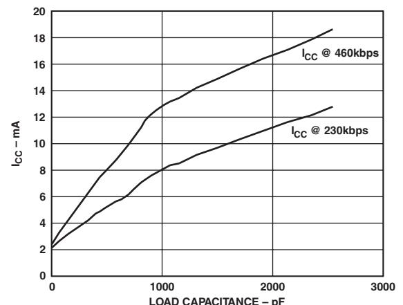
TPC 6. Power Supply Current vs. Load Capacitance
