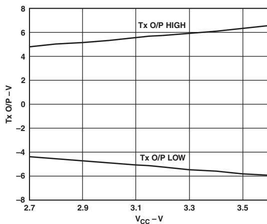
TPC 2. Transmitter Output Voltage vs. V<sub>CC</sub>
