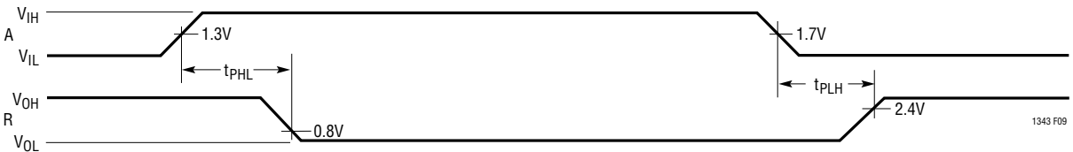
Figure 9. V.10, V.28 Receiver Propagation Delays
