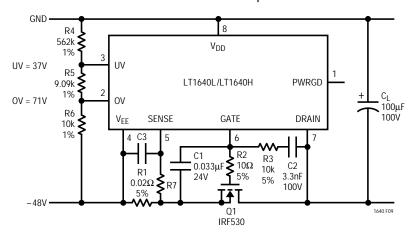
Figure 9. Extending the Short-Circuit Protection Delay
