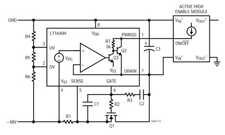
Figure 12. Active High Enable Module
