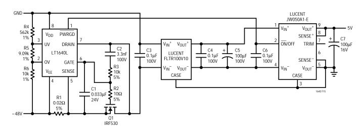
Figure 15. Typical Application Using a Filter Module
