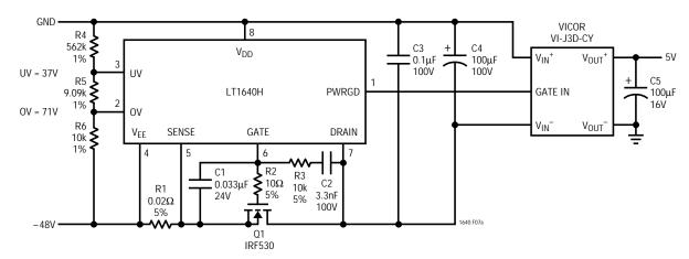
Figure 7a. Improved Inrush Control Circuitry
