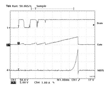
Figure 8. Short-Circuit Protection Waveforms
