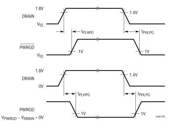
Figure 5. DRAIN to PWRGD/PWRGD Timing
