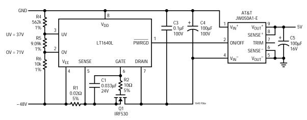
Figure 6a. Simple Inrush Control Circuitry
