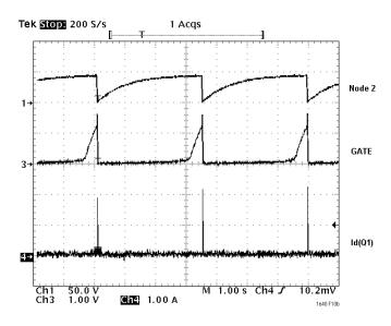
Figure 10. Automatic Restart After Current Fault
