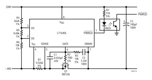
Figure 14. Using PWRGD to Drive an Optoisolator
