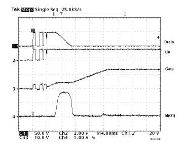
Figure 7b. Improved Inrush Control Waveforms
