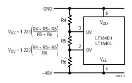
Figure 11. Undervoltage and Overvoltage Sensing
