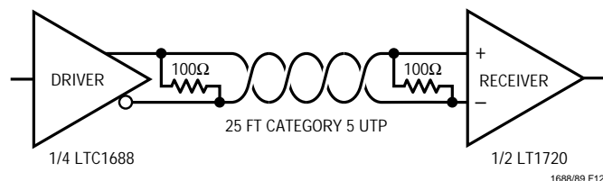
Figure 12. 100Mbps RS485 Data Connection with LT1720
