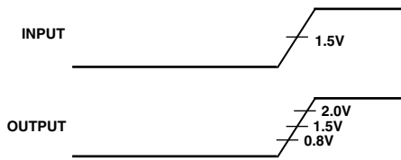
Figure 19. Voltage Reference Levels for AC Measurements (Except Output Enable/Disable)
