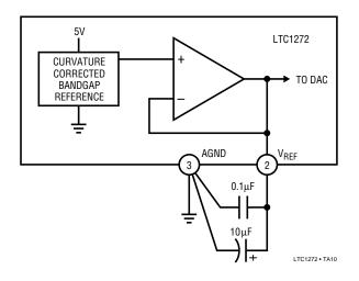
Figure 8. LTC1272 Internal 2.42V Reference
