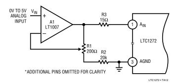
Figure 10. Unipolar OV to 5V Operation with Gain Error Adjust
