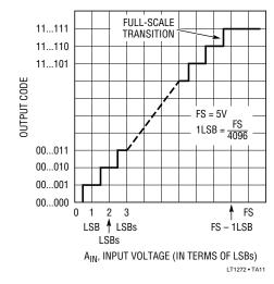
Figure 9. LTC1272 Ideal Input/Output Transfer Characteristic
