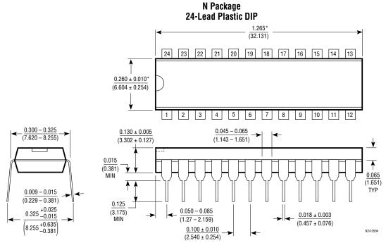
\*THESE DIMENSIONS DO NOT INCLUDE MOLD FLASH OR PROTRUSIONS. MOLD FLASH OR PROTURSIONS SHALL NOT EXCEED 0.010 INCH (0.254mm).
