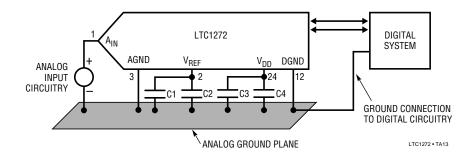
Figure 11. Power Supply Grounding Practice
