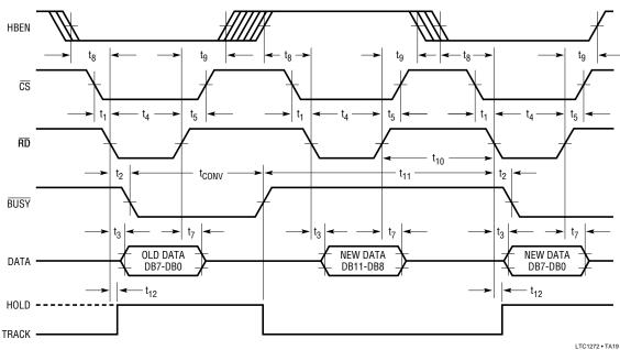
Figure 17. ROM Mode, Two Byte Read Timing Diagram
