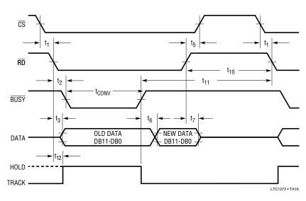
Figure 14. Slow Memory Mode, Parallel Read Timing Diagram
