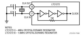
Figure 6. LTC1272 Internal Clock Circuit
