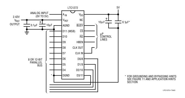
Figure 21. Single 5V Supply, 3µs, 12-Bit Sampling ADC
