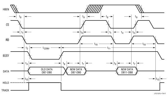
Figure 15. Slow Memory Mode, Two Byte Read Timing Diagram
