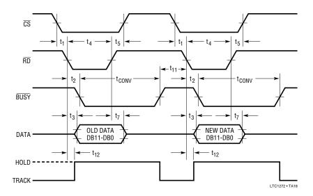
Figure 16. ROM Mode, Parallel Read Timing Diagram
