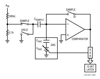
Figure 1. A<sub>IN</sub> Input
