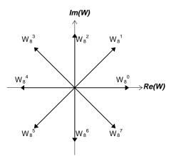
Because of the symmetry of the twiddle factor only the first four (W8<sup>0</sup>,..., W8<sup>3</sup>) must be computed.
