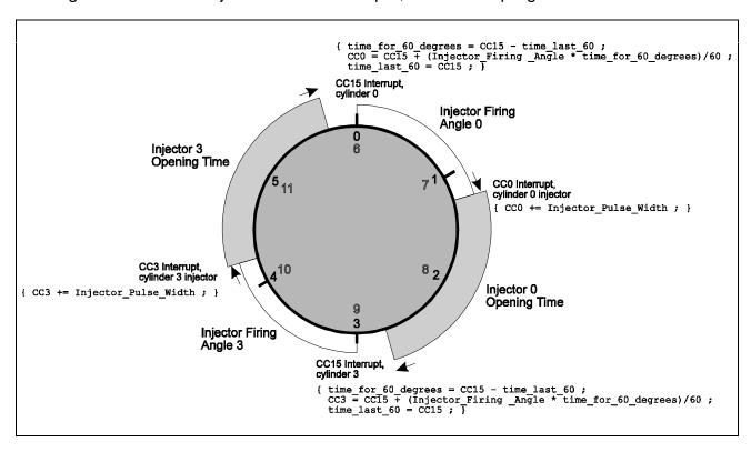
The input pulse train is fed into input capture channel 15 from a sensor giving a negative edge at each cylinder's TDC (top dead center). In a 12 cylinder engine, successive TDCs are 60 degrees apart and at the maximum operating speed of 18000rpm, this corresponds to a time of 555µs between TDC "references".
