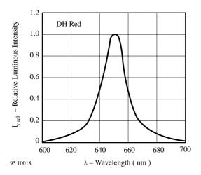
Figure 9 Relative Luminous Intensity vs. Wavelength
