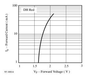
Figure 5 Forward Current vs. Forward Voltage
