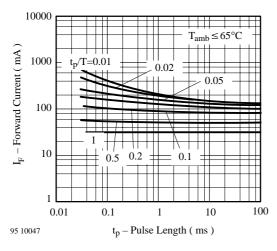
Figure 3 Forward Current vs. Pulse Length
