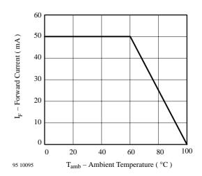
Figure 2 Forward Current vs. Ambient Temperature
