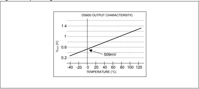
Figure 2. Output Voltage Characteristic
