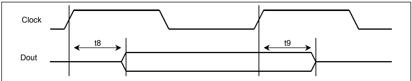
Figure 18-5. To/From Hi Z Delay Definitions (Rising Clock Edge)
