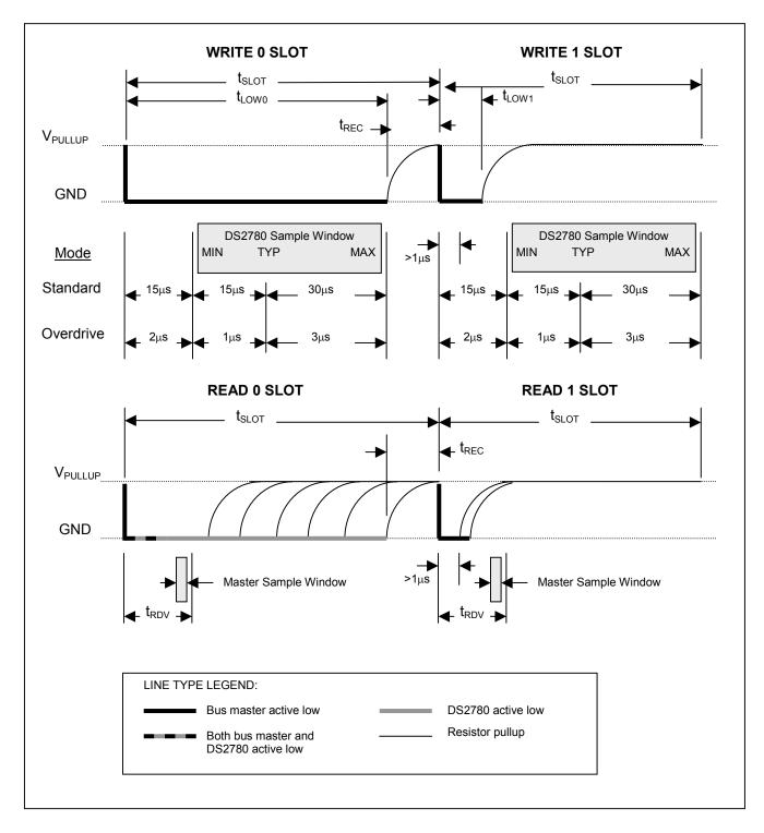
Figure 22. 1-Wire Write- And Read-Time Slots
