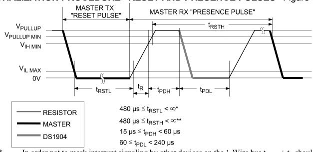
**INITIALIZATION PROCEDURE "RESET AND PRESENCE PULSES"** Figure 8
