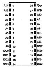
28-PIN ENCAPSULATED PACKAGE (720 Mil Extended)
