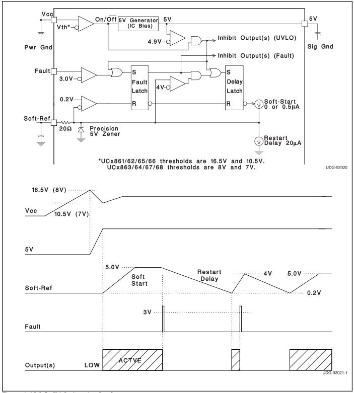
Figure 1. UVLO, 5V, fault and soft-ref.
