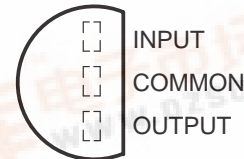
LP PACKAGE (TO-92, TO-226AA) (TOP VIEW)
