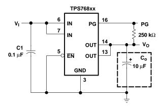
Figure 26. Typical Application Circuit (Fixed Versions)
