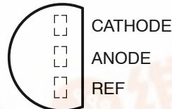
TLVH431 LP (TO-92/TO-226) PACKAGE (TOP VIEW)
