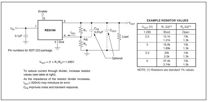
FIGURE 2. Adjustable Voltage Circuit for REG104A.
