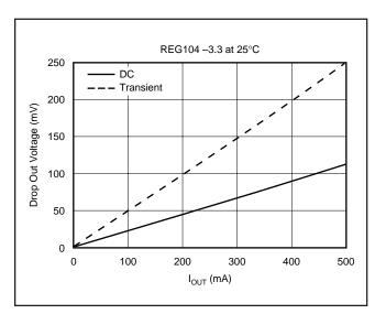
FIGURE 8. Transient and DC Dropout.
