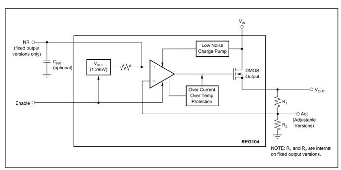
FIGURE 5. Block Diagram.
