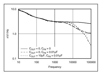
FIGURE 7. Output Noise Density on Adjustable Versions.
