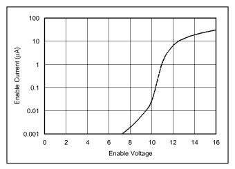
FIGURE 4. Enable Pin Current versus Applied Voltage.
