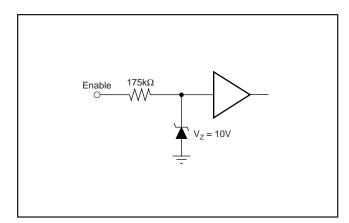
FIGURE 3. Enable Pin Equivalent Input Circuit.
