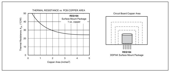
FIGURE 10. Thermal Resistance versus PCB Area for the Five-Lead DDPAK.
