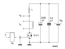
Figure 16. Unclamped Inductive Waveform
