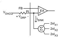
Figure 17. Load Droop Circuit
