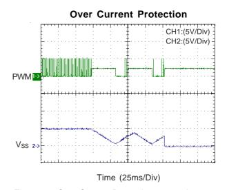
Figure 20. Over Current Protection at steady state
