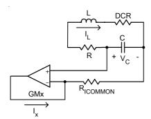
Figure 7. Current Sense Circuit
