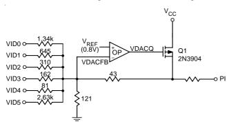
Figure 6. Immune circuit against CPU Leakage Current
