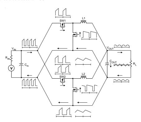
Figure 22. Power Stage Ripple Current Path
