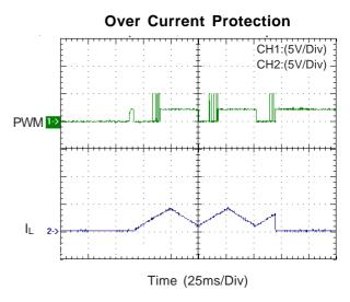
Figure 19. The Over Current Protection in the interval
