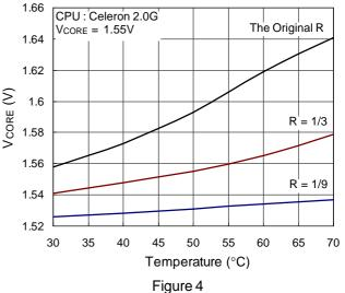
**V<sub>CORE</sub> vs. Temperature**
