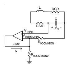
Figure 15. Application circuit of GM
