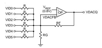
Figure 18. The Structure of Discrete DAC Generator
