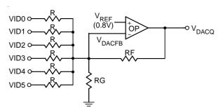
Figure 1. The Structure of Discrete DAC Generator
