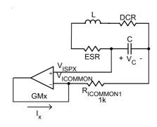
Figure 9. The Test Circuit of GM
