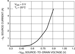
Figure 10. Diode Forward Voltage versus Current
