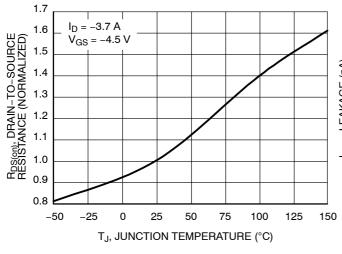
Figure 5. On–Resistance Variation with Temperature
