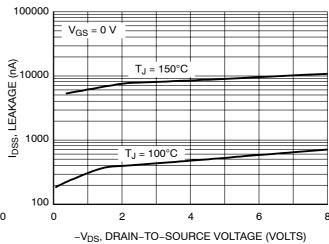
Figure 6. Drain-to-Source Leakage Current versus Voltage
