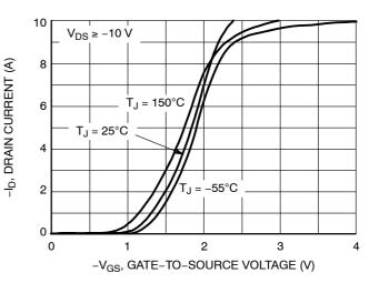
Figure 2. Transfer Characteristics
