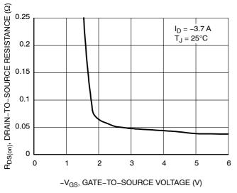
Figure 3. On-Resistance versus Gate-to-Source Voltage
