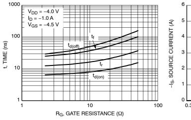
Figure 9. Resistive Switching Time Variation versus Gate Resistance
