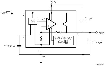
\*ON/OFF input must be actively terminated. Tie to  $V_{\mbox{\scriptsize IN}}$  if this function is not to be used.
