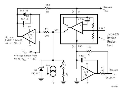
FIGURE 2. LM3420 Test Circuit
