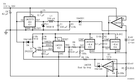
FIGURE 10. (Fast) Pulsed Constant Current 2-Cell Charger
