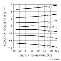
Normalized Temperature Drift with Output Externally Trimmed
