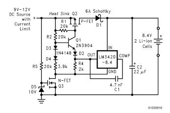
FIGURE 11. MOSFET Low Dropout Charger
