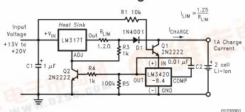
Typical Constant Current/Constant Voltage Li-Ion Battery Charger
