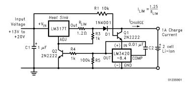
FIGURE 5. Constant Current/Constant Voltage Li-Ion Battery Charger
