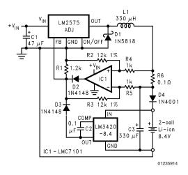
FIGURE 9. High Efficiency Switching Charger with High Side Current Sensing
