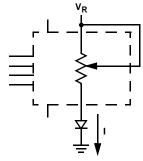
TWO-TERMINAL VARIABLE RESISTOR; VARIABLE CURRENT
