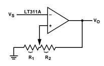
$\begin{aligned} &V_{UL} = [R_1 \, / \, (R_1 + R_2)] \, V_O(max) \\ &V_{LL} = [R_1 \, / \, (R_1 + R_2)] \, V_O(min) \end{aligned}$
