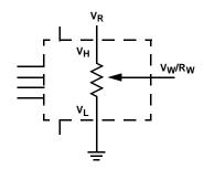
THREE-TERMINAL POTENTIOMETER; **VARIABLE VOLTAGE DIVIDER**
