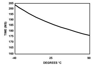
FIGURE 19. t<sub>PURST</sub> VS. TEMPERATURE
