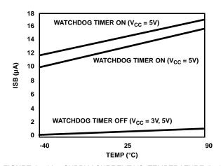
FIGURE 15.  $V_{CC}$  SUPPLY CURRENT VS. TEMPERATURE (I<sub>SB</sub>)
