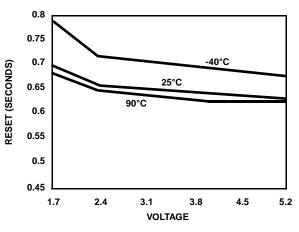
FIGURE 18. t<sub>WDO</sub> VS. VOLTAGE/TEMPERATURE (WD1, 0 = 1, 0)
