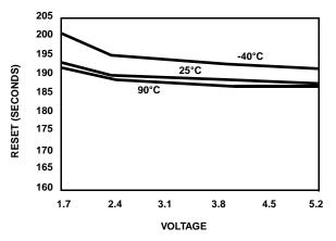
FIGURE 20. t<sub>WDO</sub> VS. VOLTAGE/TEMPERATURE (WD1, 0 0 = 0, 1)
