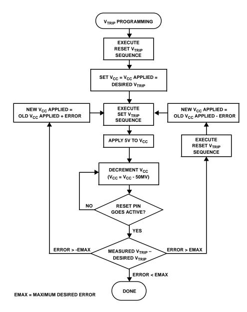
FIGURE 3. V<sub>TRIP</sub> PROGRAMMING SEQUENCE FLOW CHART
