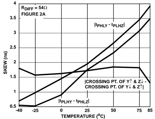
FIGURE 13. DRIVER SKEW vs TEMPERATURE (ISL83485, ISL83490, ISL83491)
