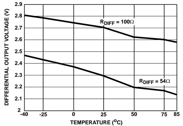
FIGURE 7. DRIVER DIFFERENTIAL OUTPUT VOLTAGE vs TEMPERATURE
