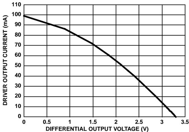
FIGURE 6. DRIVER OUTPUT CURRENT vs DIFFERENTIAL OUTPUT VOLTAGE
