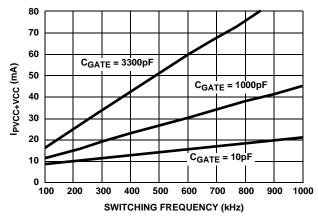
FIGURE 2. BIAS SUPPLY CURRENT vs FREQUENCY
