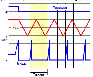
FIGURE 4. TYPICAL OVERCURRENT PROTECTION
