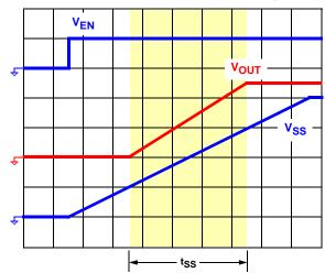
FIGURE 3. TYPICAL SOFT-START INTERVAL
