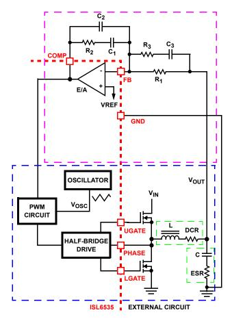
FIGURE 7. VOLTAGE-MODE BUCK CONVERTER COMPENSATION DESIGN
