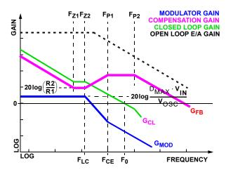
FIGURE 8. ASYMPTOTIC BODE PLOT OF CONVERTER GAIN
