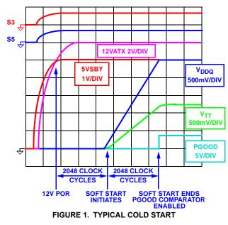
VREF\_IN pin, the S5 to S0 transition profile of the V<sub>TT</sub> rail will have a more rounded features at the start and end of the soft start whereas the V<sub>DDQ</sub> profile has distinct starting and ending points to the ramp up.
