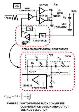
The modulator transfer function is the small-signal transfer function of V<sub>OUT</sub>/V<sub>E/A</sub>. This function is dominated by a DC Gain and the output filter (L<sub>O</sub> and C<sub>O</sub>), with a double pole break frequency at F<sub>LC</sub> and a zero at F<sub>ESR</sub>. The DC Gain of
