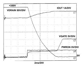
FIGURE 20. +350V LOW SIDE SWITCHING CGATE = 1000pF
