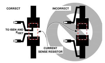
FIGURE 1. SENSE RESISTOR PCB LAYOUT
