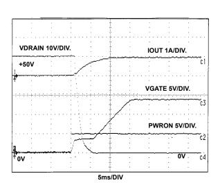
FIGURE 15. ISL6115 'HIGH' OVERCURRENT RESPONSE
