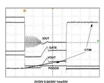
FIGURE 14. ISL6115 'LOW' OVERCURRENT RESPONSE
