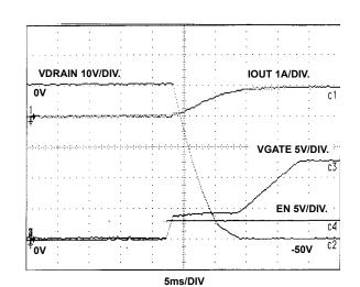
FIGURE 16. ISL6116 'HIGH' OVERCURRENT RESPONSE
