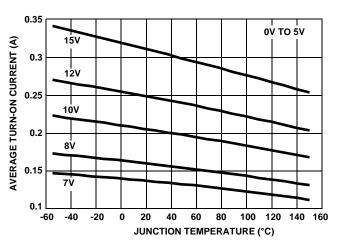
FIGURE 10. GATE DRIVER AVERAGE TURN-ON CURRENT
