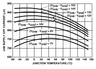
FIGURE 3. FLOATING SUPPLY OFF BIAS CURRENT
