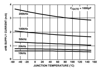
FIGURE 5. FLOATING SUPPLY SWITCHING BIAS CURRENT
