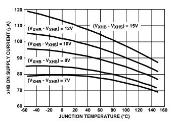
FIGURE 4. FLOATING SUPPLY ON BIAS CURRENT
