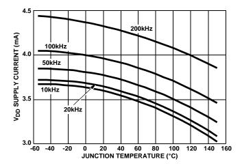
FIGURE 2.  $V_{\mbox{\scriptsize DD}}$  SUPPLY CURRENT vs SWITCHING FREQUENCY
