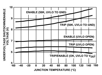
FIGURE 7. UNDERVOLTAGE THRESHOLD
