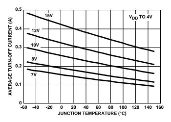
FIGURE 11. GATE DRIVER AVERAGE TURN-OFF CURRENT
