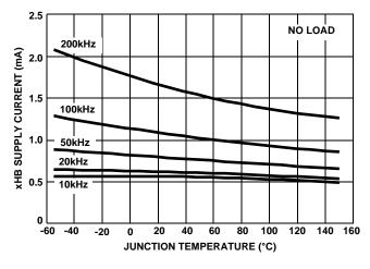
FIGURE 6. FLOATING SUPPLY SWITCHING BIAS CURRENT
