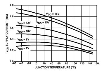
FIGURE 1.  $V_{DD}$  SUPPLY CURRENT vs  $V_{DD}$  SUPPLY VOLTAGE
